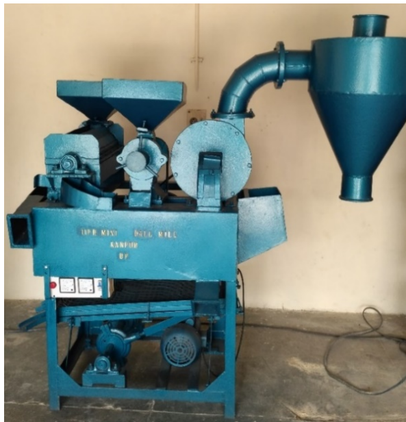
Fig.1: IIPR Mini Dal Mill (Source: Author taken, 2019)
